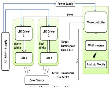
Fig. 3 System Block Diagram
