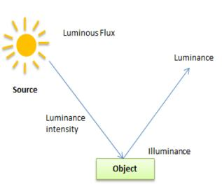
Fig. 1 Basic light terms for incident and reflected rays
