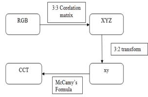
Fig. 2 Flow of CCT Calculation
