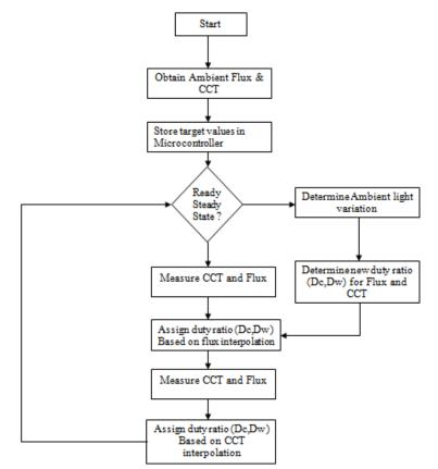
Fig.5 Flowchart for Closed loop Non-Linear system
